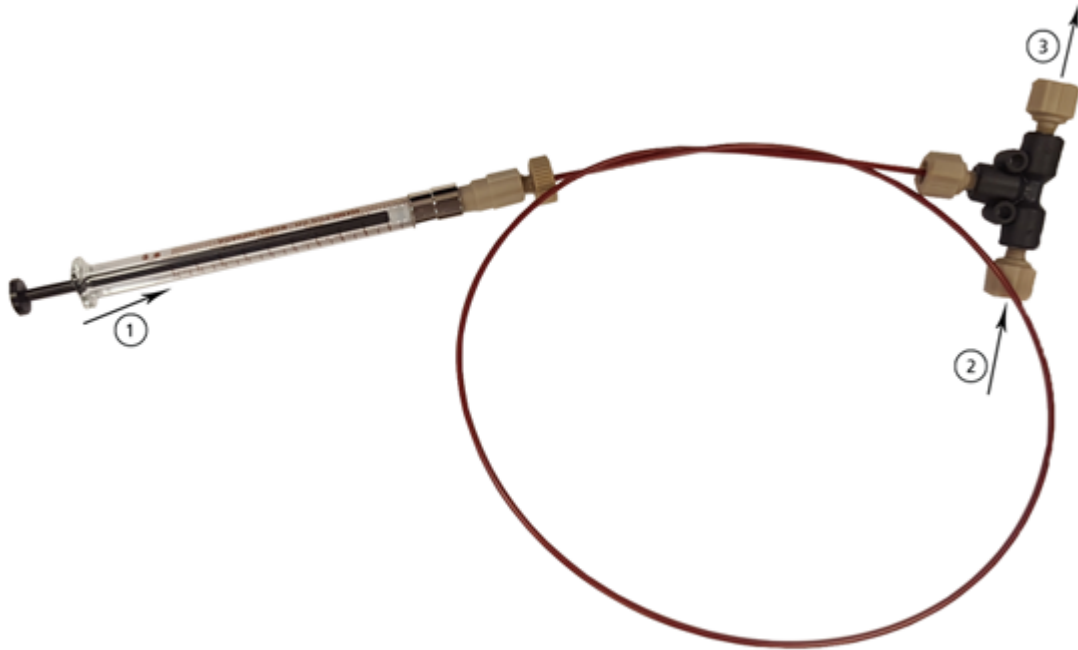
Figure 4-1 Tee Infusion Setup
