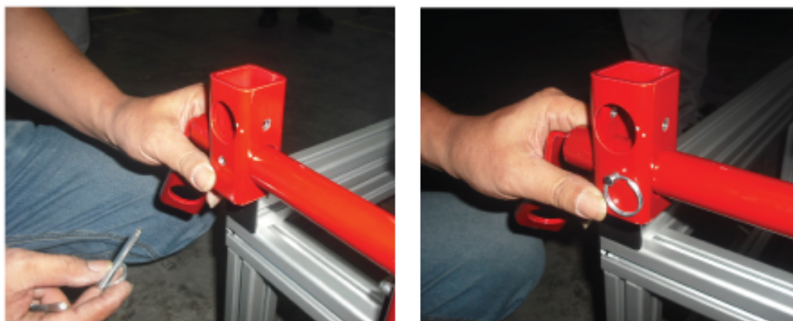
Figure 5-9 Short Block Installed
