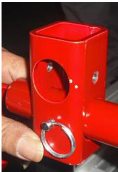
Figure 5-11 Tall Block Installed
