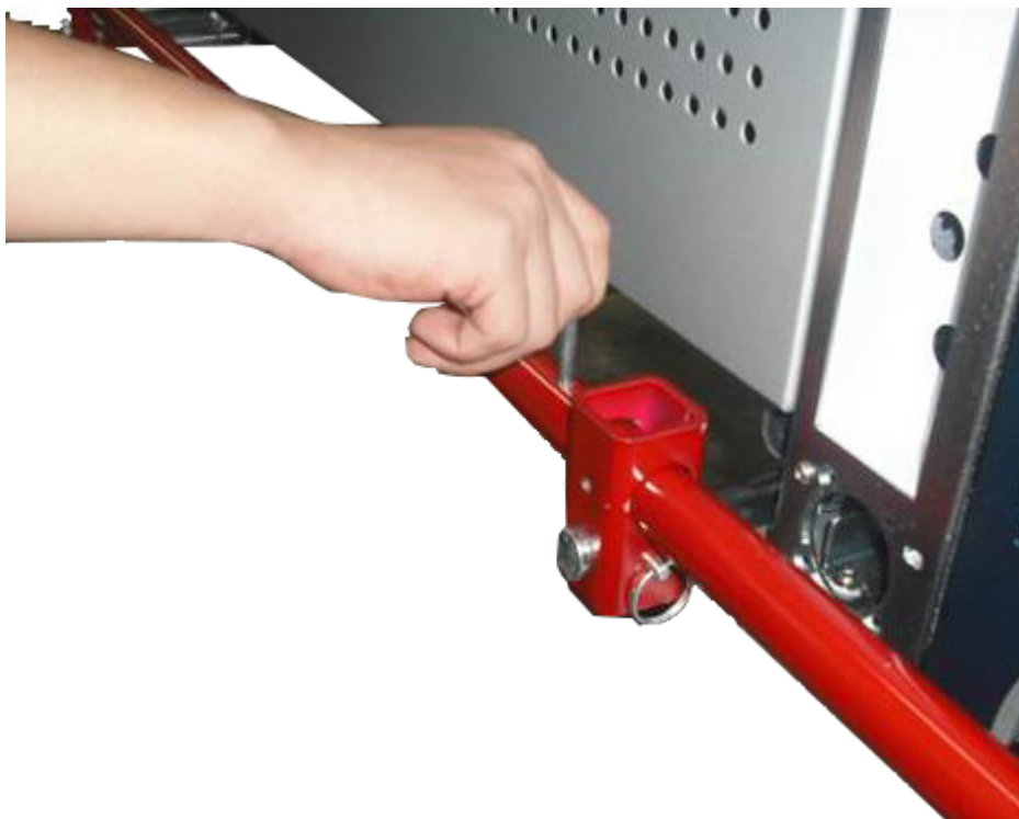
Figure 6-11 Installing the Locking Pin on the Log Rod
