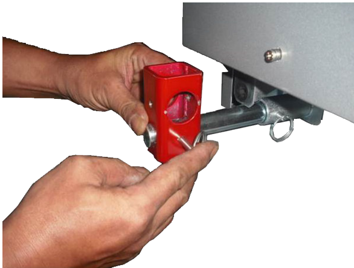
Figure 6-10 Short Block Installed
