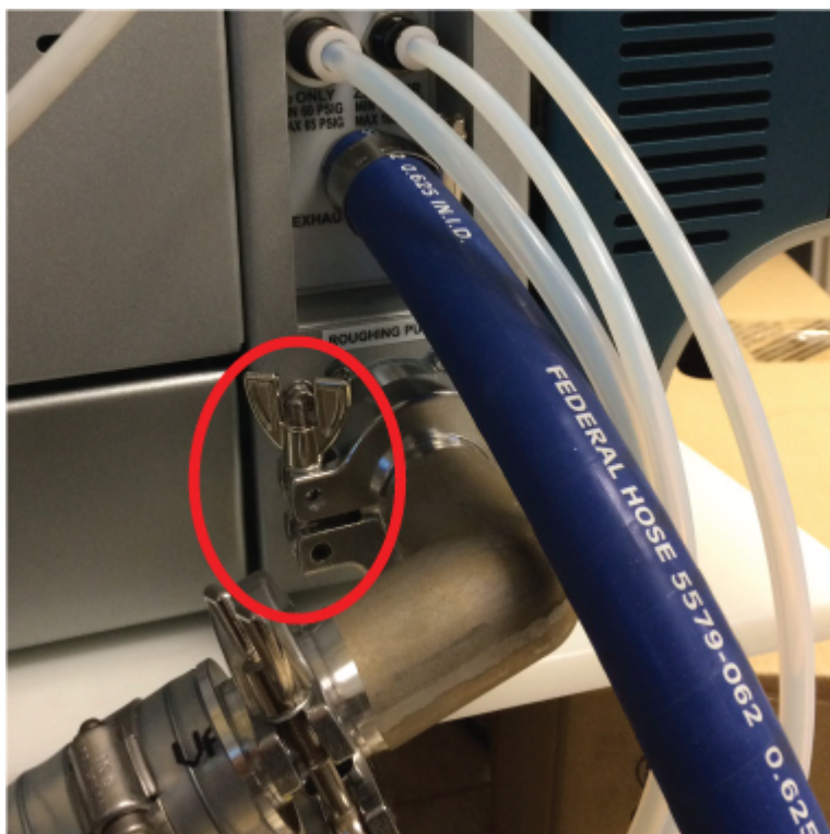
Figure 6-16 Correctly Installed Clamp
