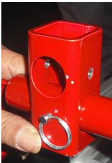
Figure 6-12 Tall Block Installed
