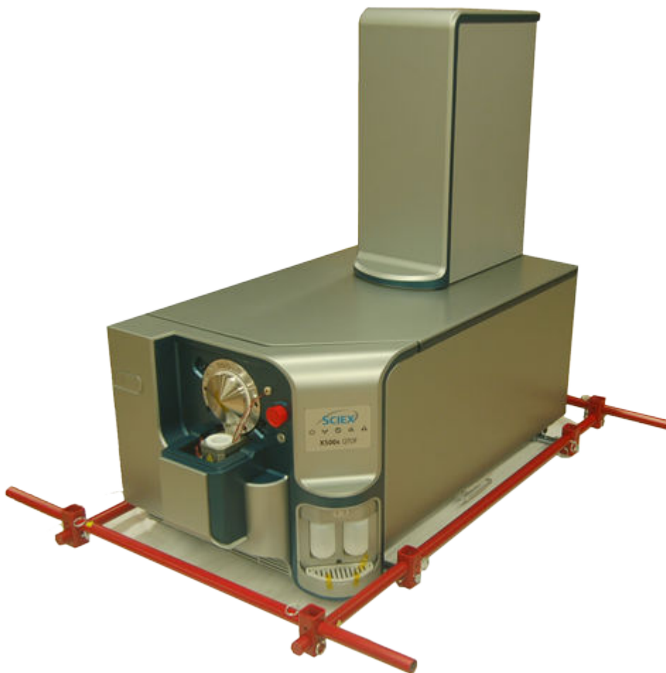
Figure 6-14 Lifting Kit Installed (X500R System)
