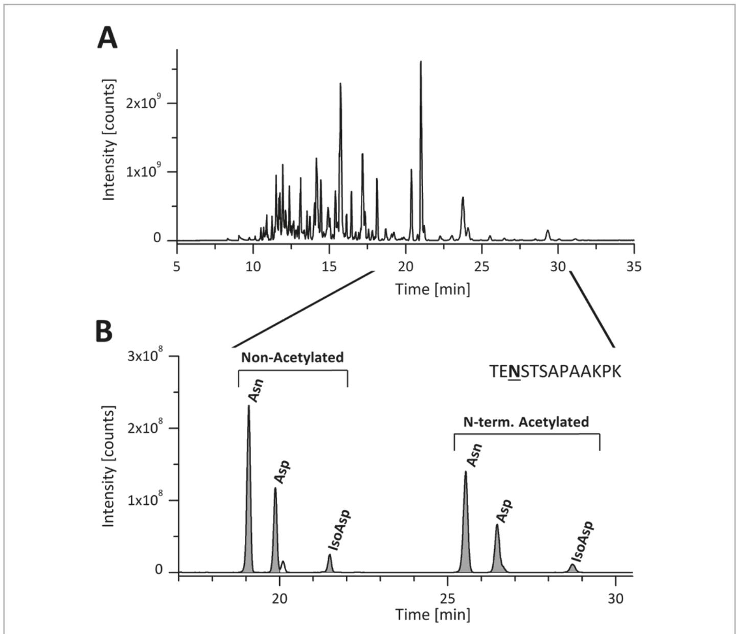
**Figure 2.** CESI-MS separation using a neutrally coated capillary (BGE 0.1 M acetic acid) of human placenta H1 histones digested with endoproteinase Arg-C. (A) Base peak electropherogram and (B) extracted ion electropherogram of deamidated and acetylated forms of the N-terminal peptide TENSTSAPAAKPK.
