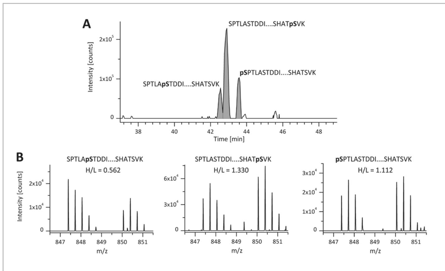
**Figure 1.** A) CESI-MS separation of 3 mono-phosphopeptide isomers of SPTLASTDDINSASASVNSHATSVK peptide detected in a fraction of a Lys-C cleaved yeast sample. B) Quantification spectra and H/L ratios of the three SILAC labeled phosphopeptide pairs.
