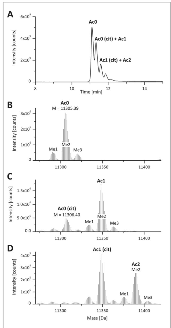
**Figure 3.** CESI-MS separation using a neutrally coated capillary (BGE, 0.1 M acetic acid) of intact citrullinated and non-citrullinated core histone H4. (A) Total ion electropherogram and (B-D) Mass deconvoluted spectra of individual H4 peaks.
